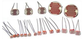
Light Dependent Sensor (Resistance changed by light)
